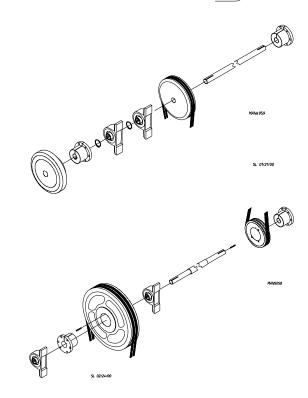
Tighten cap screws progressively. There should remain a gap between the sheave hub and the flange of the bushing.
